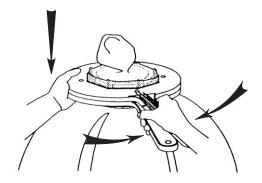
4. When the opening of the expander is centered over the collar lower the expander until the mouth of the balloon is lower than the bottom of the collar ring.
