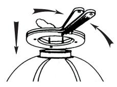
3. Make sure the prongs are upward and the opening of the expander is directly over the collar of the machine.
