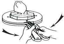
2. Simply squeeze the handles together and the prongs will spread apart stretching the balloons to fit over the machine collar.
