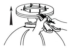
Squeeze the handles together so the prongs expand to their maximum. Lift the expander over and off the collar. The balloon is now loaded on the stuffing machine.
