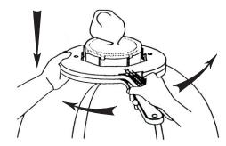
5. Releasing the pressure on the handles of the expander will allow the balloon to fit closely to the collar. Make sure the mouth of the balloon is below the bottom of the tabs on the collar. With a downward motion push the expander until the balloon releases from the prongs of the expander.
